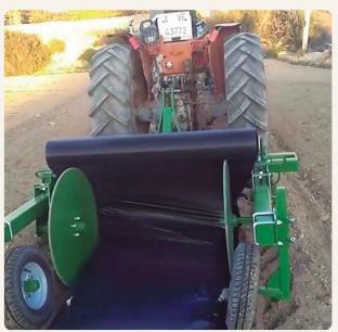
The STF mulching machine was created and adapted by FORIGO ROTER ITALIA specifically for the application of AgroPaper® mulch, either on one and two furrows simultaneously.
