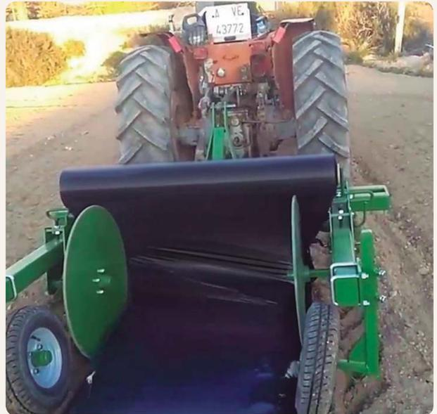
The STF mulching machine was created and adapted by FORIGO ROTER ITALIA specifically for the application of AgroPaper® mulch, either on one and two furrows simultaneously.
